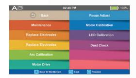
① Select [Maintenance] in [Maintenance Menu] ② Execute [Maintenance], then the following checks will be made.
