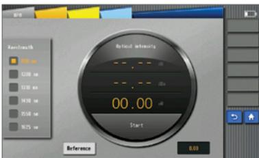
OPM is used for measuring the absolute optical power meter or relative optical power loss through the span of the optical fiber.
