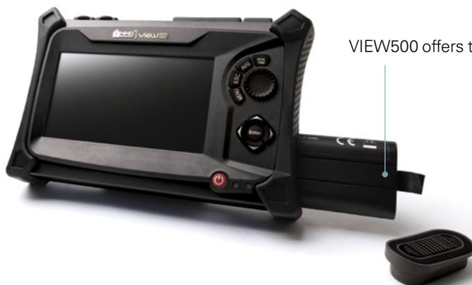
VIEW500 offers the ultra-high battery capacity of 7800mAh.
