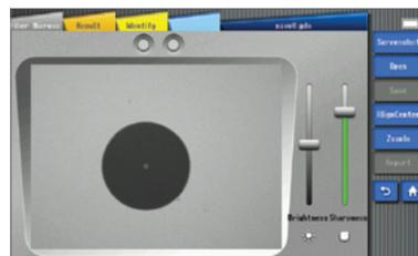
Fiber end tester (peripheral required) is mainly used to test the cleanliness and flatness of the fiber end face.
