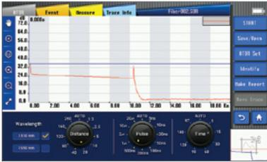
OTDR mode allows for measuring distance, loss, reflectivity, attenuation and accumulation loss on a fiber optic link.
