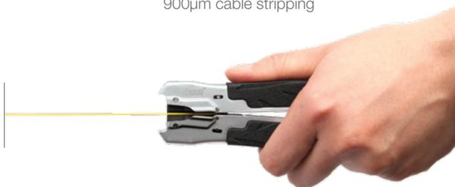
After stripping 900µm, stripping 250µm
