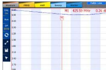
Cable Loss measures inherent loss of the RF cable (displayed in log scale).
