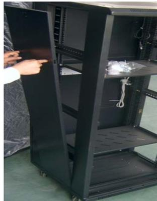
**2.10:** Chucking the clips to the middle of side panels by two hands, and then pushing the side panel to frame;
