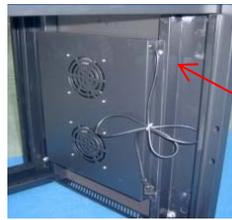
**2.3:** Using the tapping screws M5x10 to fix the fan tray under the top;
