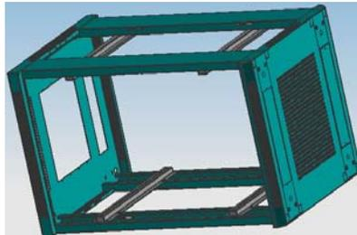
**2.4:** Installing the bayonet-type nut M6 on the frame; and then using the allen screw M6x10 to connect the mounting angle and frame tightly;
