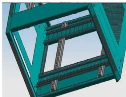
**2.5:** Installing the bayonet-type nut M6 on the mounting angle; and then using the allen screw M6x10 to connect the mounting profile and mounting angle;
