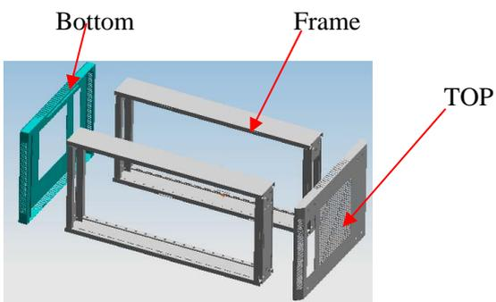
**2.1:** Putting the frame to top and bottom together, which must be alignment to frame. Using the hex socket set screws M8x12 to fix them.
