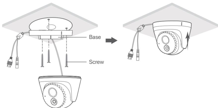
**3 B. Run the cable through the bottom**
