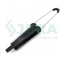
This wedge type anchor clamp is consists of main body, wedges, thimble, plastic insert, 2.5mm stainless steel bail wire, aluminum bail head. All the plastic parts are made of UV resistant plastic which processed by injection technology and aluminum bail head was processed by CNC machine which is available in Jera workshop.
