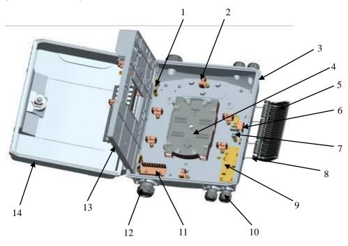
Picture 2: Inner layer structure (Same for A and B type)
