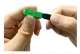
Put down tail clip, tighten screw cap, and install the housing.
