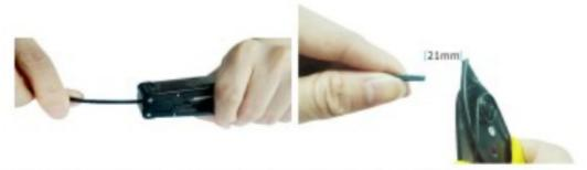
③ Stripe the covered wire, ④ Stripe fiber coating, stripped length 50mm keep 21mm
