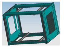
2.4: Installing the bayonet-type nut M6 on the frame; and then using the allen screw
