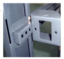
2.5: By the allen screw M6x10 to fix the spacer on the mounting angle;
